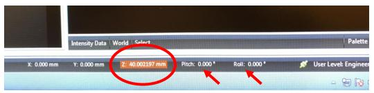
5) Turning the **Z-motion joystick very carefully when z < 10 mm.** For a standard Silicon wafer (1 mm thick), you should see the sample image becomes clear when z < 7 mm. At z ~3mm, the image becomes very clear. For thick sample, please use (thickness +2) mm as a reference.
