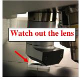
6) Keep lowering the lens carefully using **SLOW** mode. Stop lens movement right after the image passes sharp focus plane and becomes slightly blurring. Press **flashing Z-STOP** button on the panel to set up **Z-STOP**. The **Z-STOP** light should be in **stable red**.
